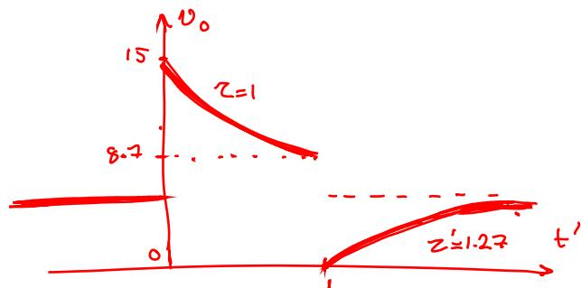
$$t > 1 \quad \begin{array}{l} v_0 = 5 - \frac{6.3}{1.27} e^{-\frac{t-1}{1.27}} \\ v_0(1^+) = 5 - \frac{6.3}{1.27} \approx 0 \end{array}$$
