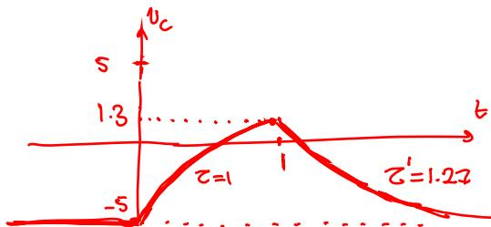
$$0 < t < 1 \quad \begin{array}{l} v_0 = 5 + 10 e^{-t} \\ v_0(0^+) = 15 \\ v_0(1^-) = 8.7 \end{array}$$
