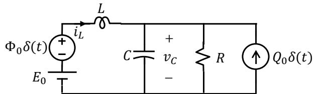
$$\begin{aligned} \text{KVL: } & \left\{ \begin{array}{l} E_0 + \Phi_0 \delta t = L \frac{di_L}{dt} + v_C(t) \\ Q_0 \delta t + i_L(t) = C \frac{dv_C}{dt} + \frac{v_C}{R} \end{array} \right. \quad (*) \\ \text{KCL: } & \left\{ \begin{array}{l} \Phi_0 = L[i_L(t) - i_L(0)] \rightarrow i_L(t) = \frac{\Phi_0}{L} + \frac{E_0}{R} \\ Q_0 = C[v_C(t) - v_C(0)] \rightarrow v_C(t) = \frac{Q_0}{C} + E_0 \end{array} \right. \quad (\dagger) \end{aligned}$$
